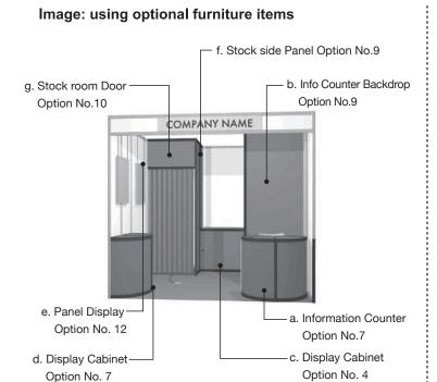
System panels are basically plywood panels with PVC vinyl color sheet finish.
